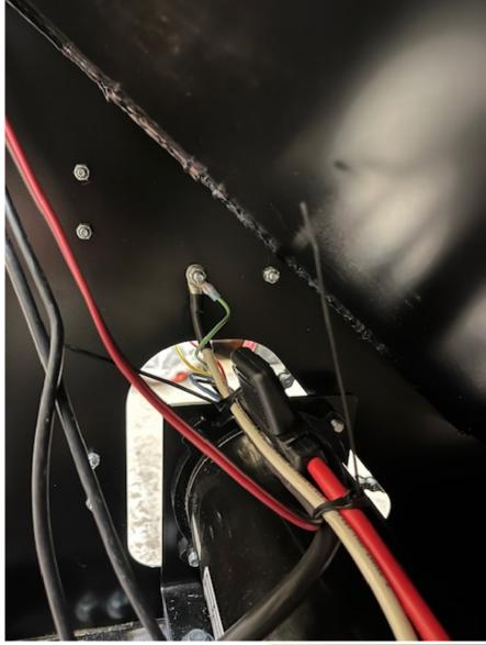
You can use the same bolt that your motor ground is attached to for the green gound wire
